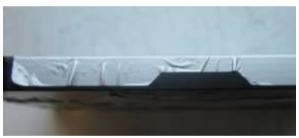
Upon discovery of tamper evidence, the module should be removed from service.
