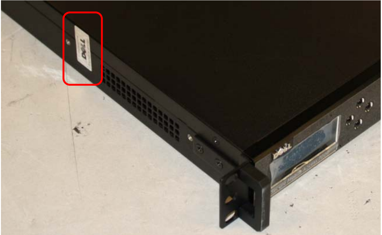
Figure 2 - Tamper Seal #1 –Chassis Seam
