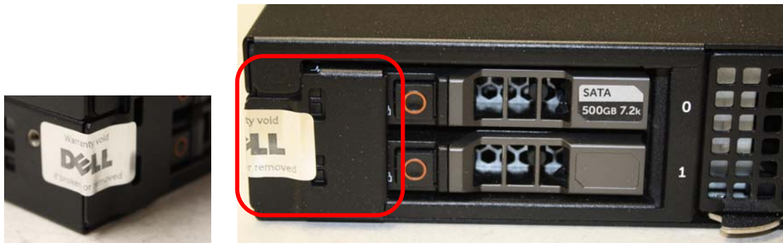
Figure 3 - Tamper Seal #2 – Tamper seal over drive bay protective plate
