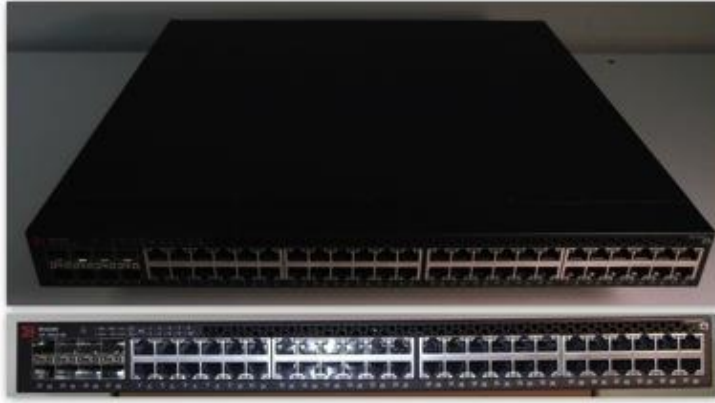
Figure 17 - Front and top side of the Brocade ICX 6610-48
