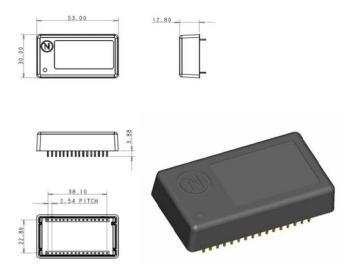
nShield Edge is a stand alone security module consisting of a fitted MiniHSM cryptographic module, a smart card reader and a USB interface integrated in a single package, as shown in the figure below.
