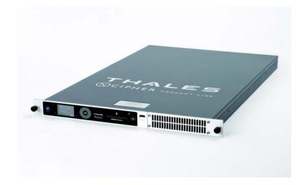
The nShield Hardware Security Modules are defined as multi-chip embedded cryptographic modules as defined by FIPS PUB 140-2.
