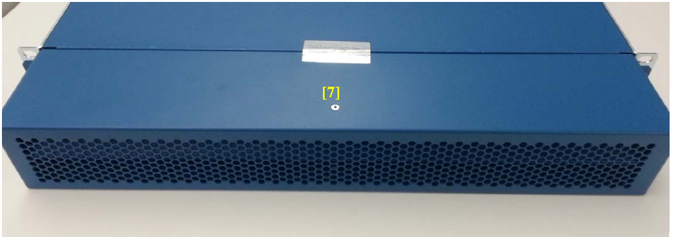
Figure 11 – PA-3060 Front/Top Tamper Seal Placement
