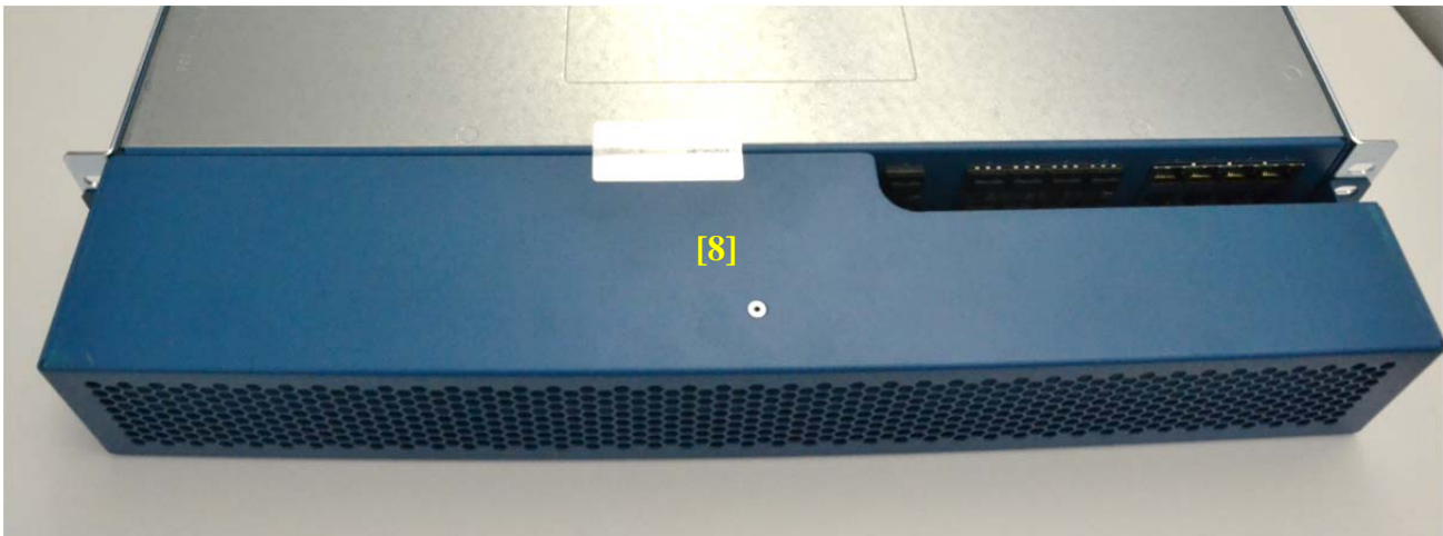
Figure 12 – PA-3060 Front/Bottom Tamper Seal Placement
