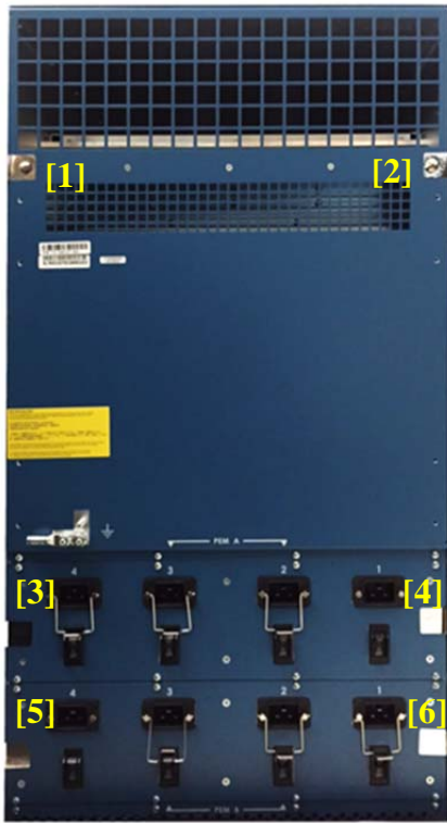
Figure 13 - PA-7080 Tamper Seal Placement for Rear (6)
