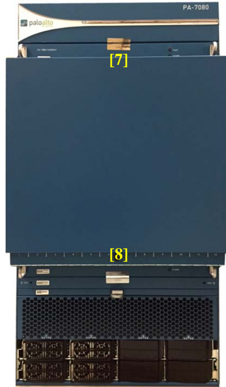
Figure 14 - PA-7080 Tamper Seal Placement on Front Fan Trays(2)
