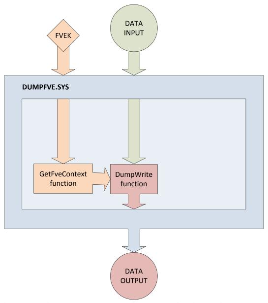
(DUMPFVE.SYS) component. A Full Volume Encryption Key (FVEK) is one of the required inputs.
