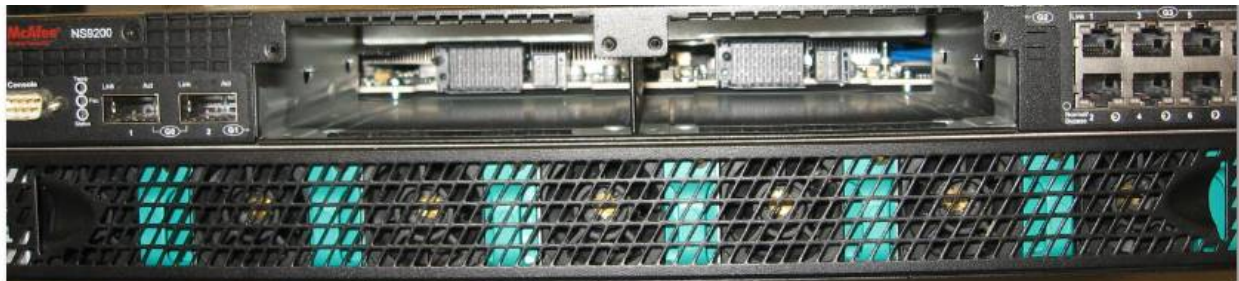
Figure 4 - Front panel with no Network I/O Modules or cover plate
