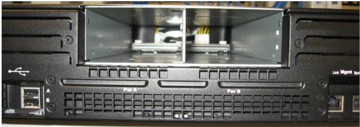
Figure 6 - Rear Panel with Power Supplies Removed
