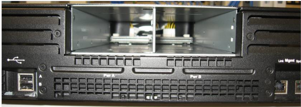
Figure 6 - Rear Panel with Power Supplies Removed
