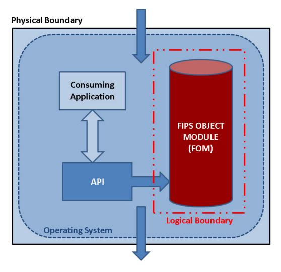
Figure 1 – FOM block diagram
