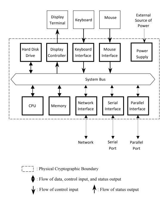
Figure 1: Cryptographic Module Hardware Block Diagram
