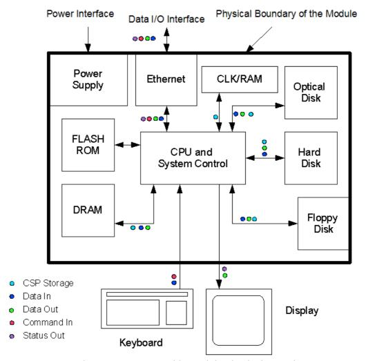
Figure 2: Cryptographic Module Physical Boundary
