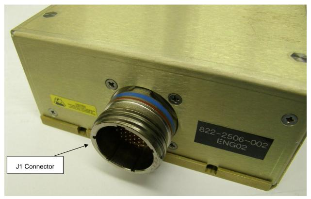
Figure 7 DVP-200 Rear Apron (Showing J1 Connector)
