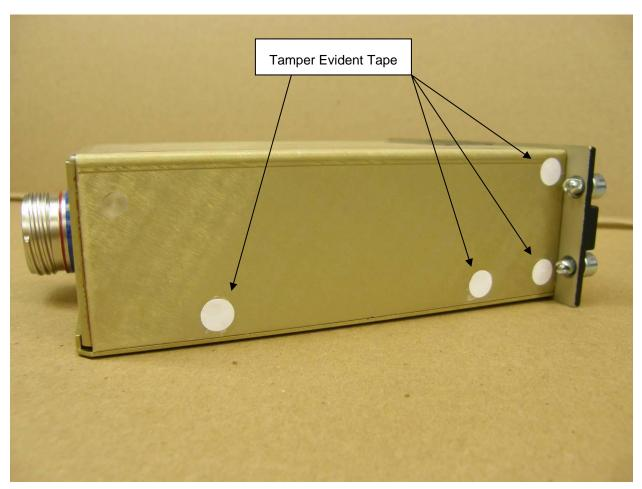
Figure 10 DVP-200 Tamper Evident Tape Right Side
