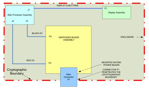
Figure 1 - DVP-200 Cryptographic Boundary
