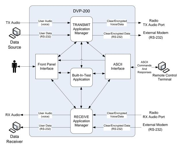
Figure 6 DVP-200 Block Diagram
