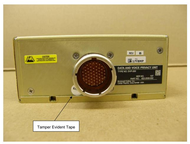
Figure 12 DVP-200 Tamper Evident Tape Rear
