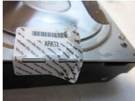
Figure 5: Tamper Evidence on Metal Surface
