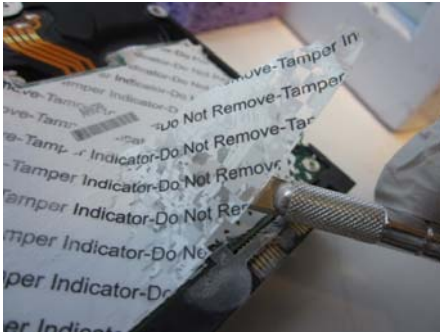
Figure 4: Tamper Evidence on Large Tamper Label
