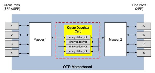
Figure I - The Module on Circuit Pack for Secure Communication
