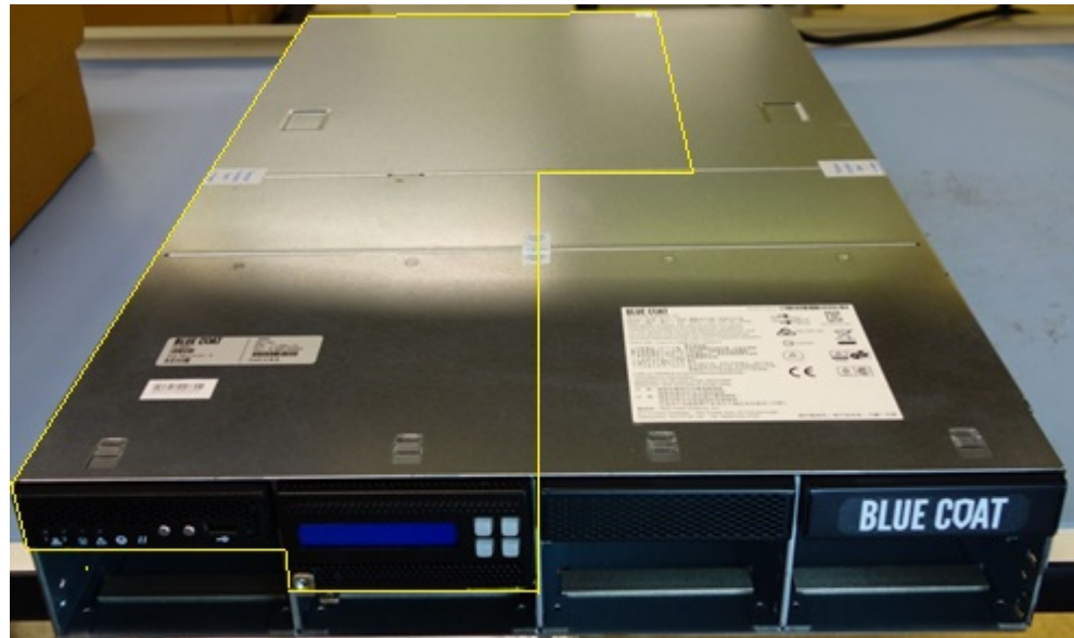
Figure 2–10 SV3800 Cryptographic Boundary Definition
