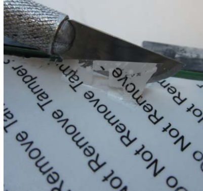
Figure 3: Tamper Evidence on Tamper Label
