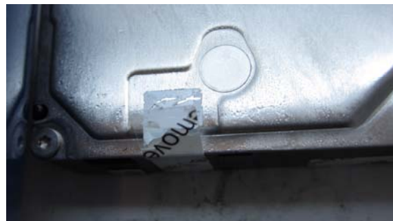
Figure 5: Tamper Evidence on Metal Surface
