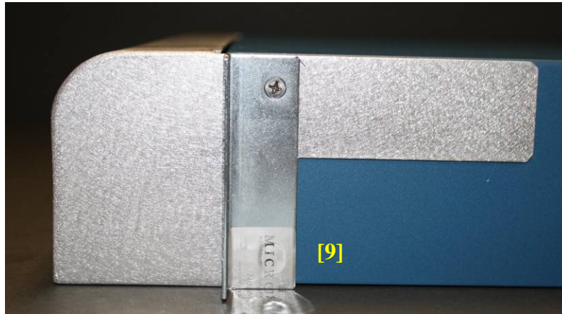
Figure 40 - PA-4000 Series Right Side Tamper Seal Placement (1)
