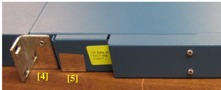
Figure 36 - PA-3000 Series Tamper Seal Placement (2)
