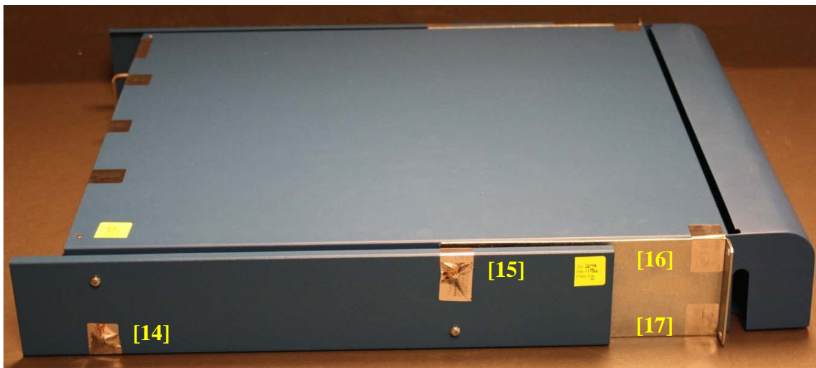
Figure 44 - PA-5000 Series Left Side Tamper Seal Placement (4)
