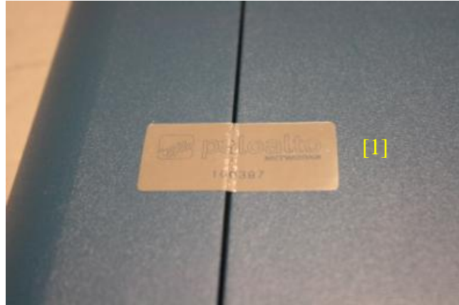
Figure 27 - PA-500 Front Tamper Seal Placement (1)
