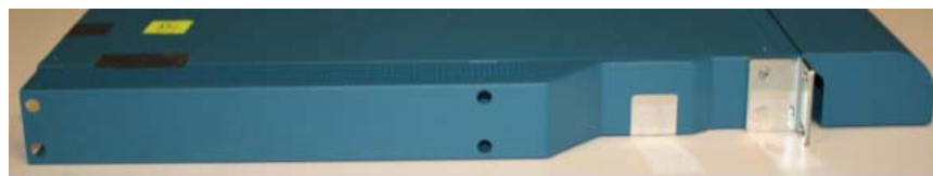
Figure 11 - PA-2020 / PA-2050 with Side Opacity Shield
