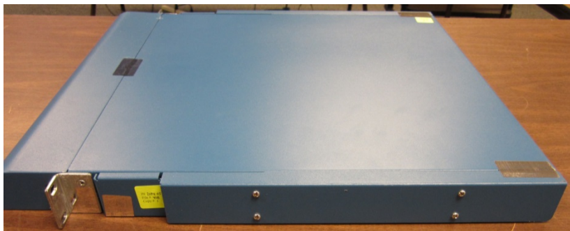
Figure 15 - PA-3020 / PA-3050 side with Opacity Shield
