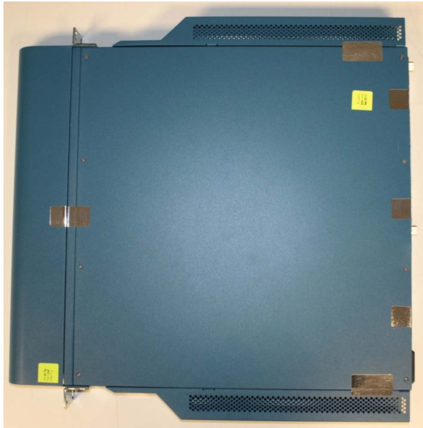
Figure 10 - PA-2020 / PA-2050 Front Opacity Shield
