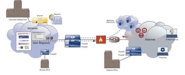
Figure I Typical Deployment of a ProxySG 9000 Series Appliance
