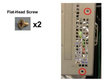
Figure 8 Small Louver Alignment
