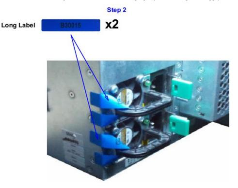
Figure 10 Tamper-Evident Labels for Power Supplies
