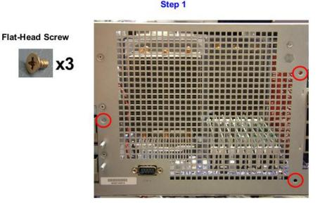
Figure 7 Large Louver Alignment
