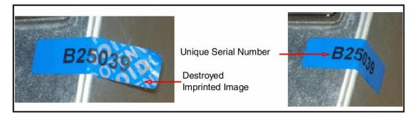
Figure 9 Label Showing Tamper-Evidence
