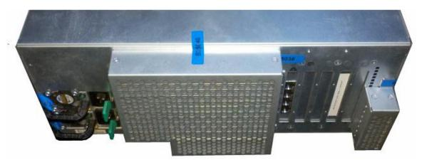
Figure 6 Installed Louvered Shutters and Tamper-Evident Labels
