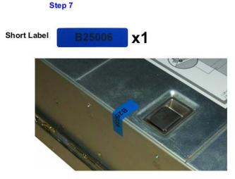
Figure 14 Tamper-Evident Label Application - Top and Side of Appliance
