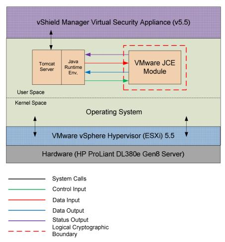
Figure 3 - VMware JCE Module Logical Cryptographic Boundary
