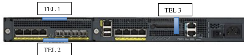
Figure 26 Cisco ASA 5550 Security Appliance Tamper Evident Label Placement. This unit is identical to ASA 5510, 5520 and 5540 above as far as TEL placement. The 5550 image is provided because it has additional ports on the front. All other sides are similar to ASA 5510, 5520 and 5540
