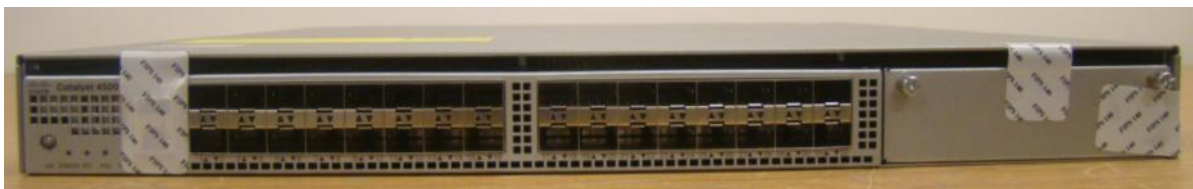
Figure 17 - C4500X-32SFP+ / C4500X-F-32SFP+ (three TELs on front)
