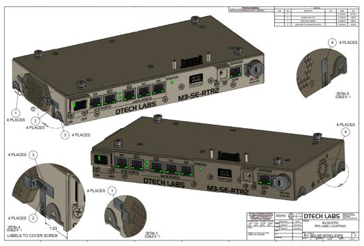
Figure 6: M3-SE-RTR2-FIPS Tamper Evidence
