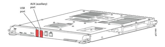
Figure 6: EX8216-RE320 Tamper-Evident Seal Location—Chassis Front
