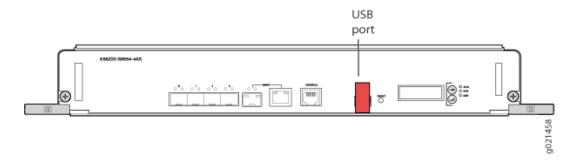
Figure 4: EX6210-SRE64-4XS Tamper-Evident Seal Location—Routing Engine Front
