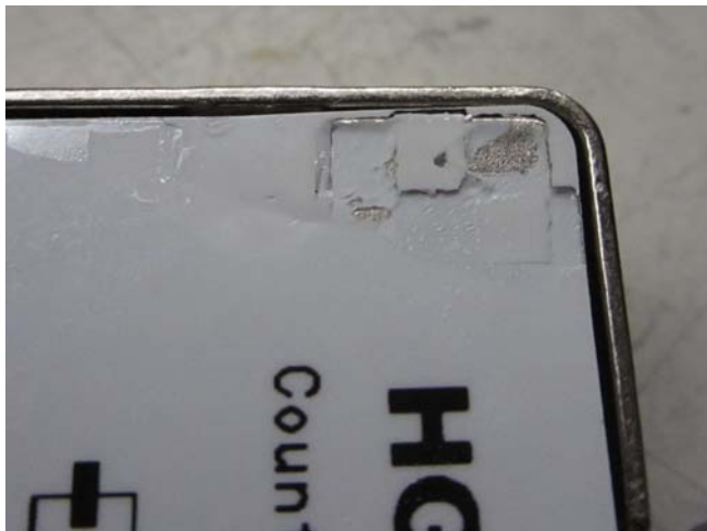
Figure 4: Tamper Evidence on Large Tamper-Evident Label
