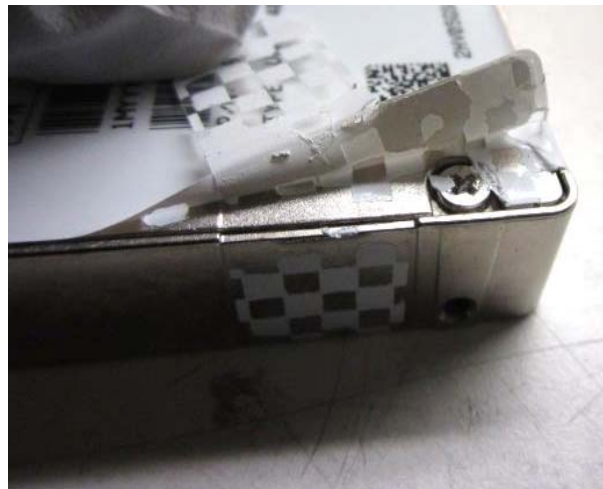
Figure 5: Tamper Evidence on Smaller Tamper-Evident Label
