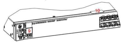
Figure 16 - OOBM and Top Panel Tamper-Evidence Label Placement (24-port Switch)
