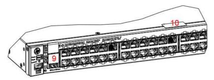
Figure 17 - OOBM and Top Panel Tamper-Evidence Label Placement (48-port Switch)
