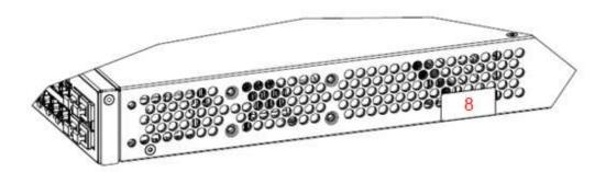
Figure 15 - Right-Hand Side Tamper-Evidence Label Placement
