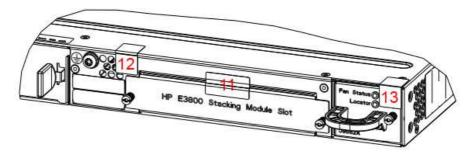
Figure 18 - Rear of Switch Tamper-Evidence Label Placement
