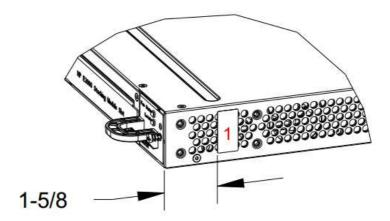
Figure 13 - Left-Hand Side Vent Openings Tamper-Evidence Label Placement (Step I)
