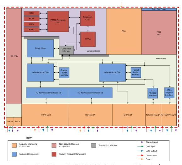
Figure 2 - HP Networking 3800 Switch Series Cryptographic Boundary9
