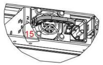
Figure 20 - Power Supply Tamper-Evidence Label Placement
