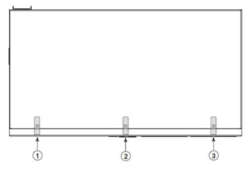
Figure 17 Top view of a Brocade ICX 6450-48 device with security seals
