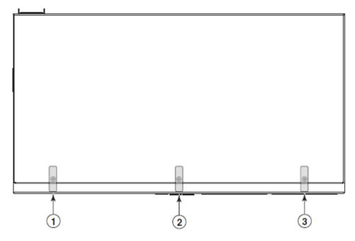
Figure 11 Top view of a Brocade ICX 6430-48P device with security seals
