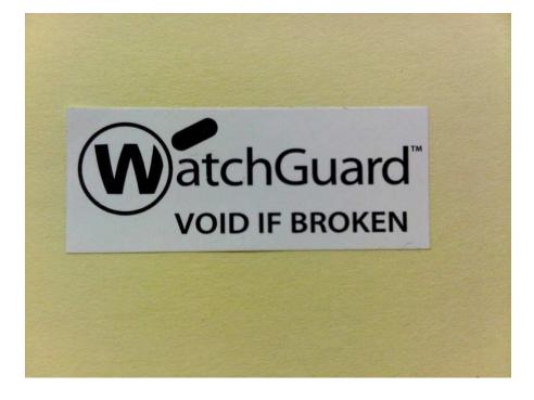
Figure 3: WatchGuard XTM Tamper Evident Label
