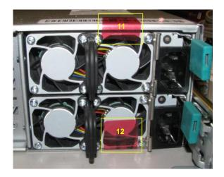
Figure 19 - Tamper-Evident Seal Application Positions (S5032/S6032 - Rear)
