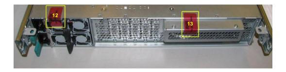
Figure 20 - Tamper-Evident Seal Application Positions (S5032/S6032 - Bottom Rear)
