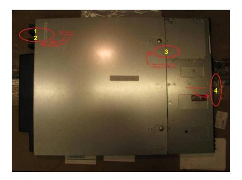
Figure 16 - Tamper-Evident Seal Application Positions (S4016)
