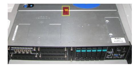
Figure 18 - Tamper-Evident Seal Application Position (S5032/S6032 - Top)
