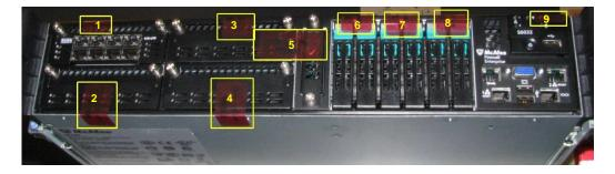
Figure 17 - Tamper-Evident Seal Application Positions (S5032/S6032 - Front)
