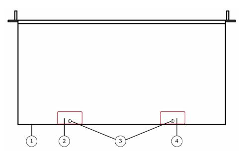
Figure 14 – Tamper-Evident Seal Application Positions (S1104)
