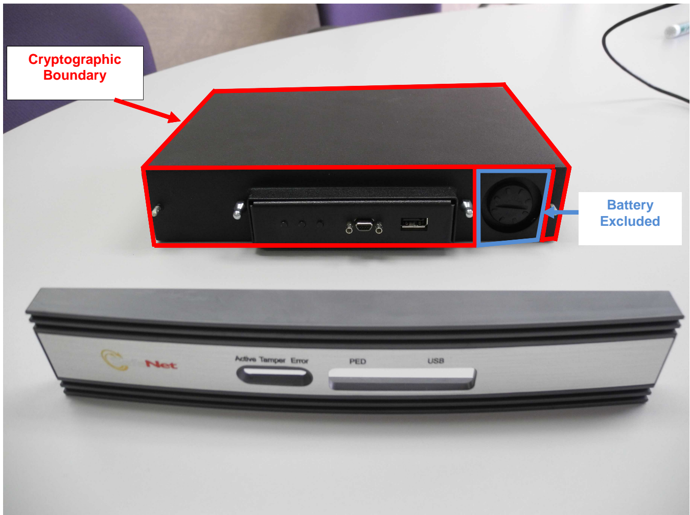
Figure 2-2. Luna G5 Cryptographic Boundary (with front bezel removed)
