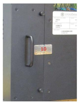
Figure 10 – X60 Tamper Evident Label Placement – Back
