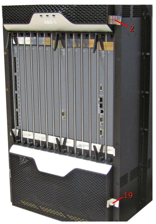
Figure 12 - X80-S Tamper Evident Label Placement - Right
