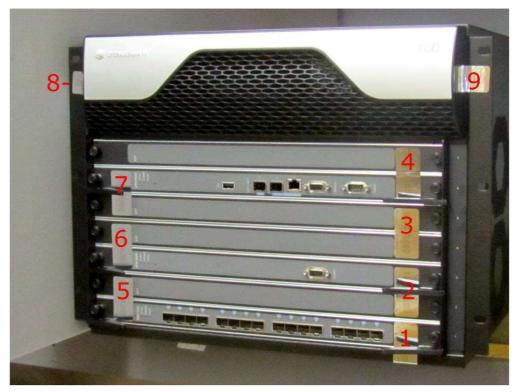
Figure 9 - X60 Tamper Evident Label Placement - Front
