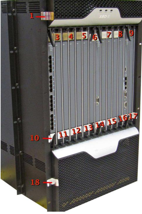
Figure 11 – X80-S Tamper Evident Label Placement – Left
