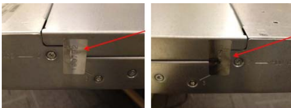
Figure 10 – Tamper-Evidence Labels on Side of ESKM
