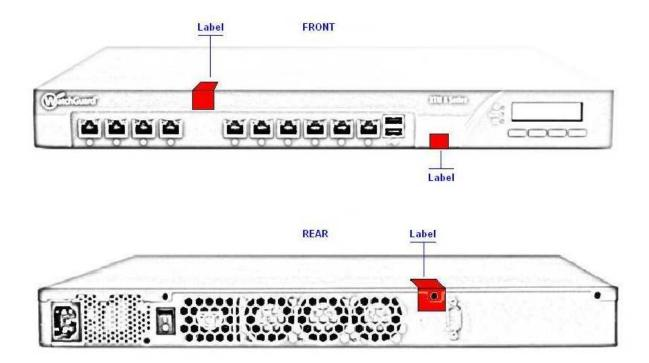
Figure 23: WatchGuard XTM 8 Series Tamper Evident Label Placement
