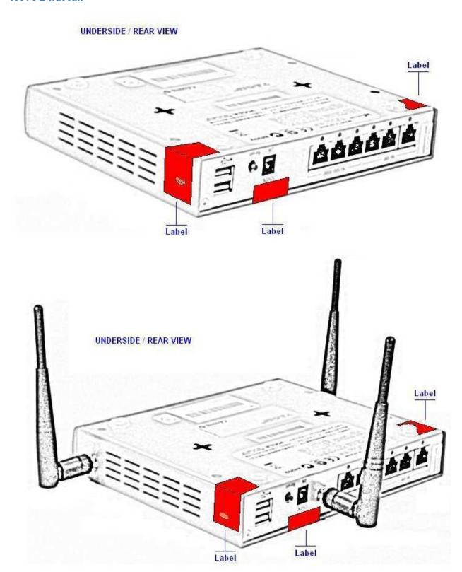
Figure 18: WatchGuard XTM 2 Series Tamper Evident Label Placement
