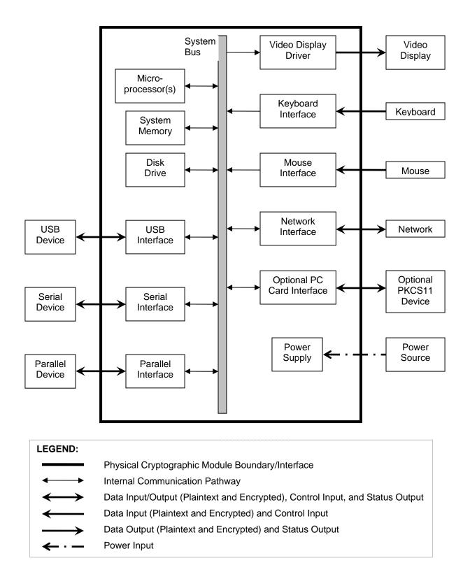
Figure 1: Cryptographic module block diagram for hardware (Physical).
