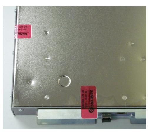
Figure 7 – Factory installed tamper seals
