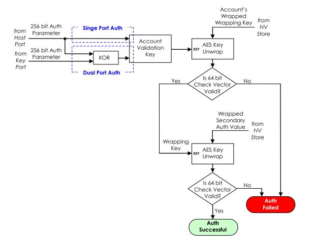
Figure 12 - Authentication Mechanism
