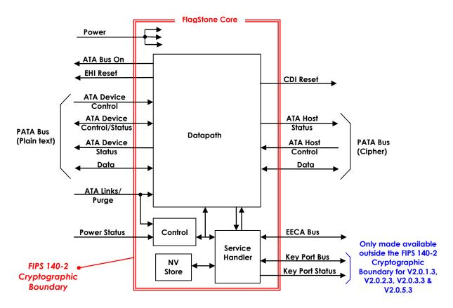
Figure 10 - FlagStone Core Simplified Block Diagram
