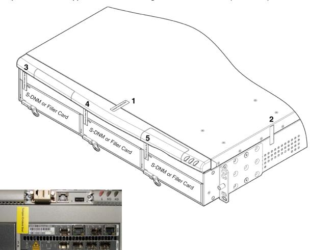
Figure 2-3 Tamper-evident seals applied to the front and right sides of the chassis (5 locations)
