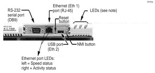
*Note:* The LEDs provide (from left to right): Shelf status, PSU B, and PSU A.
