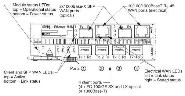
*Note:* Client ports 1, 2, 3, 4 are Small Form-factor Pluggable (SFP) client ports. WAN ports 1 and 2 support 10/100/1000Base-T (RJ-45) and 2x1000Base-X SFP.
