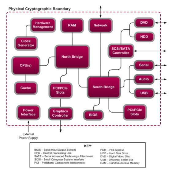
Figure 4 – Standard GPC Block Diagram
