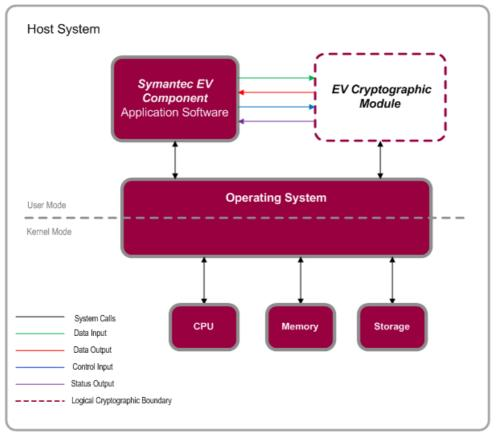
Figure 5 – Logical Block Diagram and Cryptographic Boundary
