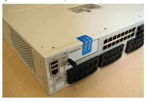
Figure 8: FortiGate-1240B AMC faceplate seal
