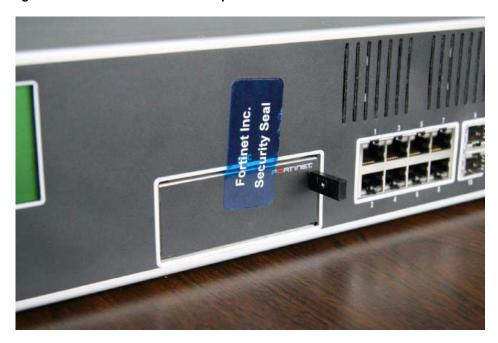
Figure 12: FortiGate-3600A AMC faceplate seal
