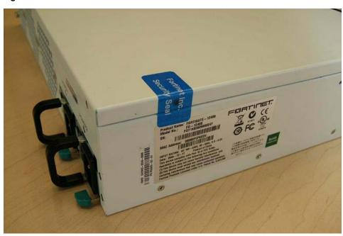
Figure 6: FortiGate-1240B external enclosure seal
