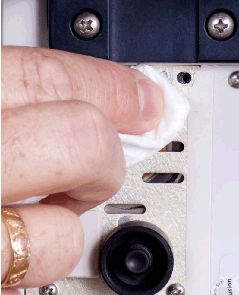
Figure 23 Removing remaining debris
