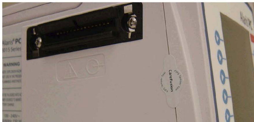
Figure 17 Affix a seal on each side of the device
