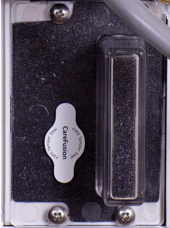
Figure 7 Ensure seal covers entire viewing hole
