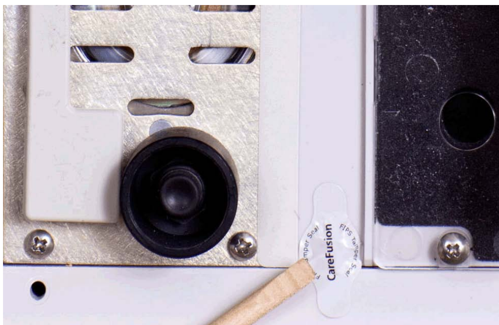
Figure 10 Ensure seal covers entire head of screw
