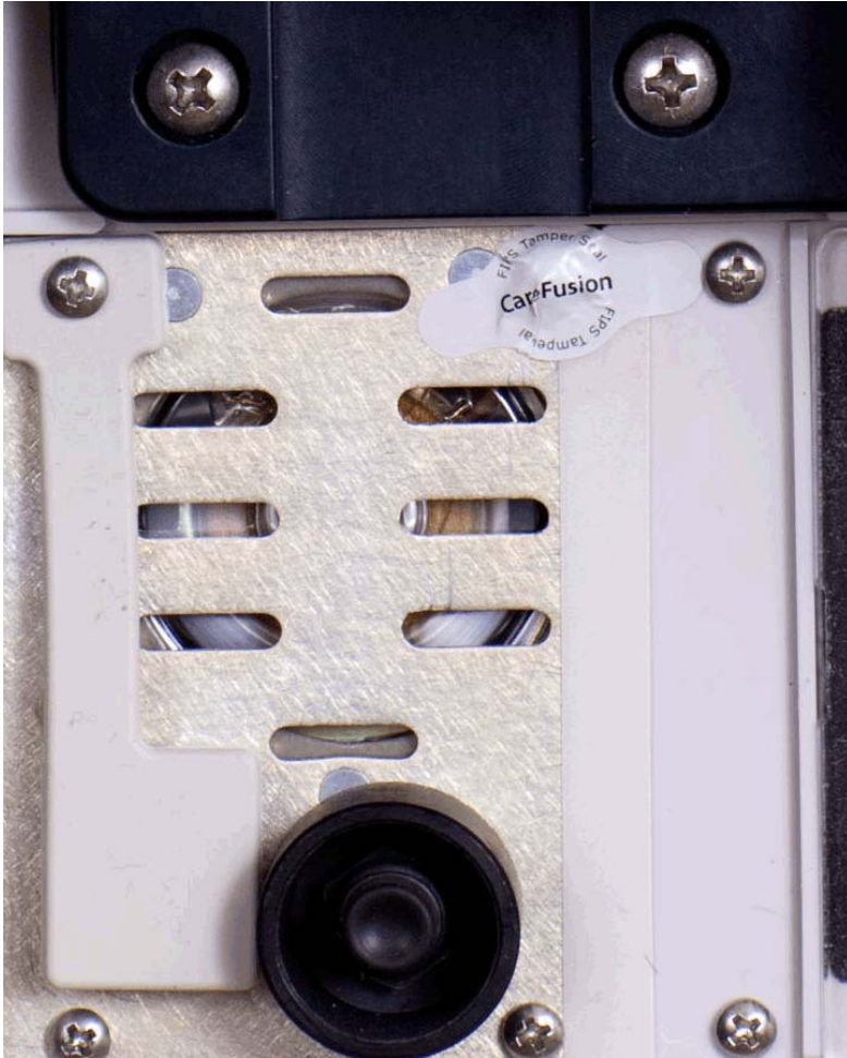
Figure 4 Seal must cover entire head of screw
