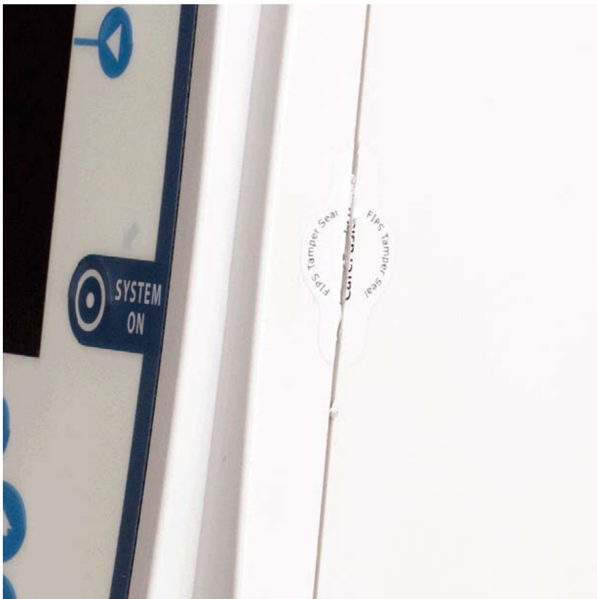
Figure 27 Seal has been sliced through
