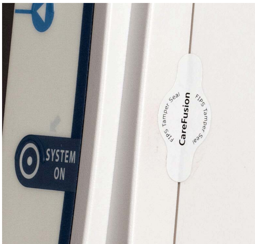
Figure 18 Ensure seal is centered between grooves
