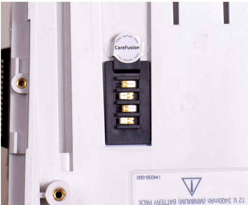
Figure 15 Ensure seal covers entire head of screw
