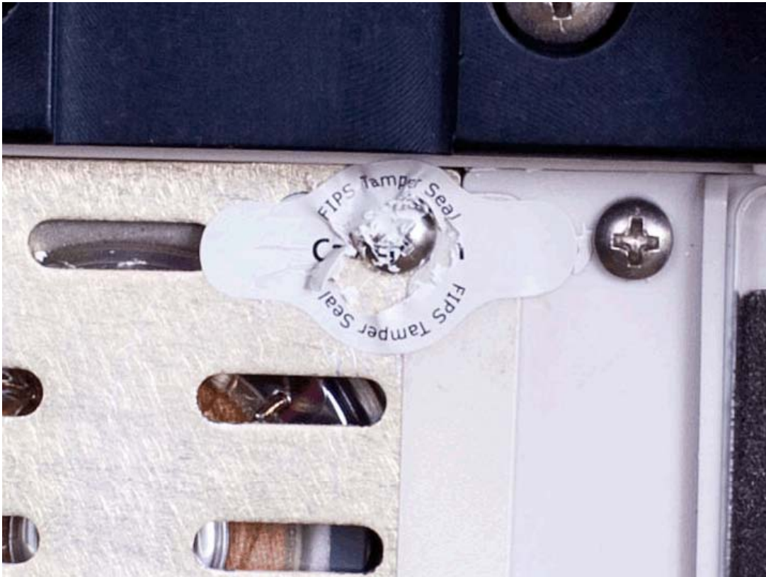
Figure 28 Seal has been gouged out
