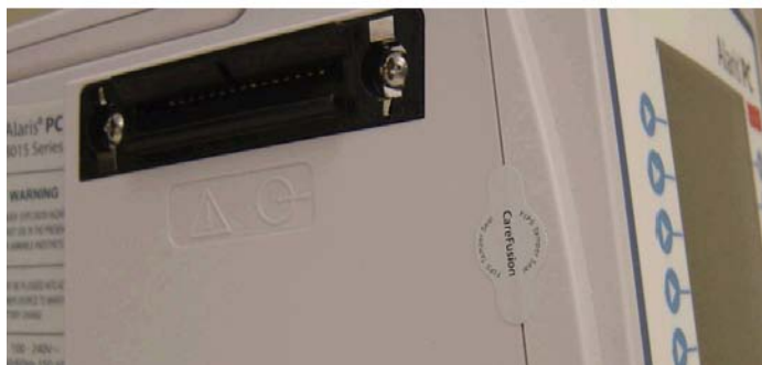
Figure 2 Location of seals on device
