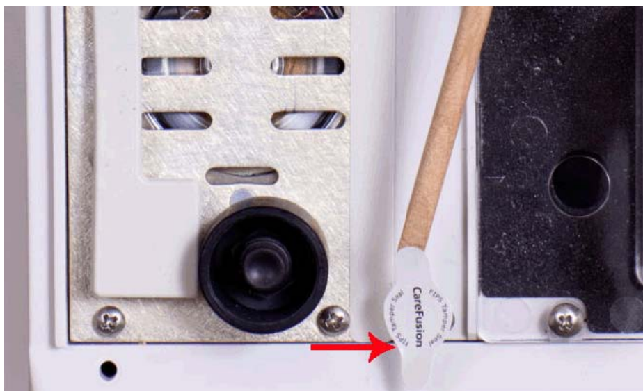
Figure 9 Affix seal over bottom screw
