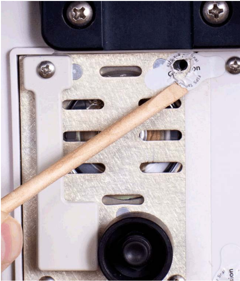
Figure 22 Use orange stick to remove debris
