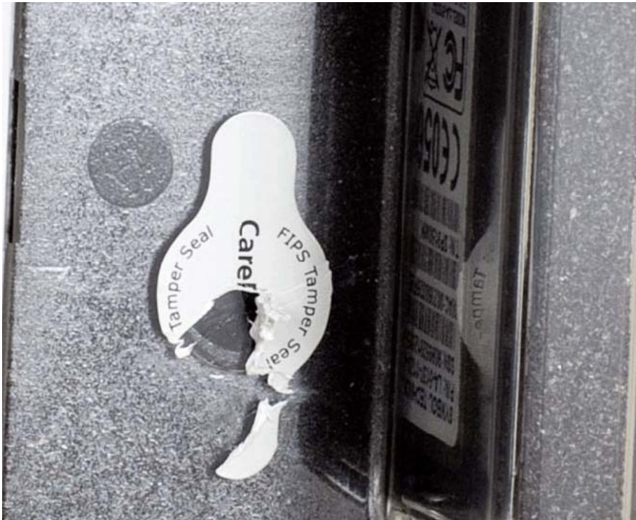
Figure 29 Seal has been partially peeled off from the device
