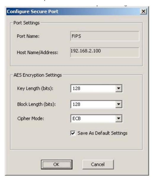
Figure 6 - Configuring a Secure Port
