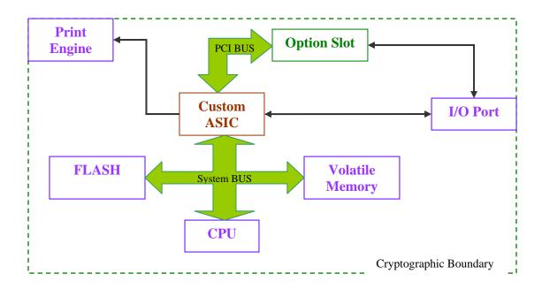
Figure 5 - Physical Cryptographic Boundary
