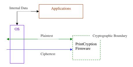
Figure 4 - Logical Cryptographic Boundary
