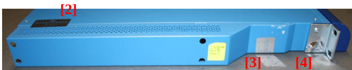
Figure 18 - PA-2000 Series Left Side Tamper Seal Placement (3)
