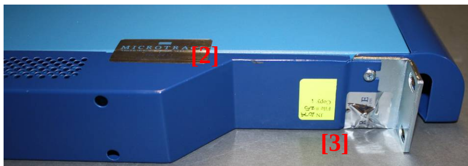
Figure 14 - PA-500 Left Side Tamper Seal Placement (2)
