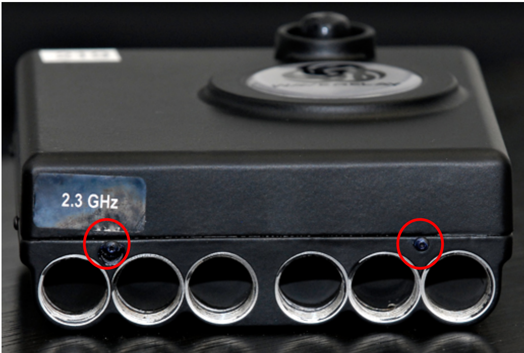
Figure 3 – Tamper-evident material placement for MPU Bottom (2 locations indicated by red circles)
