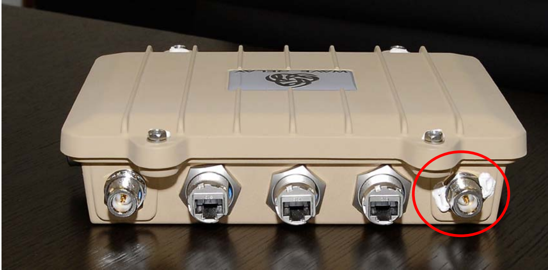
Figure 5 – Tamper-evident material placement for Quad Radio Router Wireless Radio Port (Top – 2 locations indicated by the red circle)
