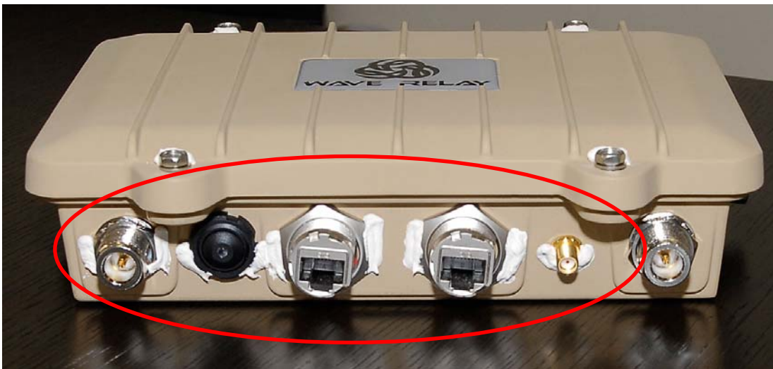
Figure 6 – Tamper-evident material placement for Quad Radio Router Bottom (9 locations indicated by the red circle)
