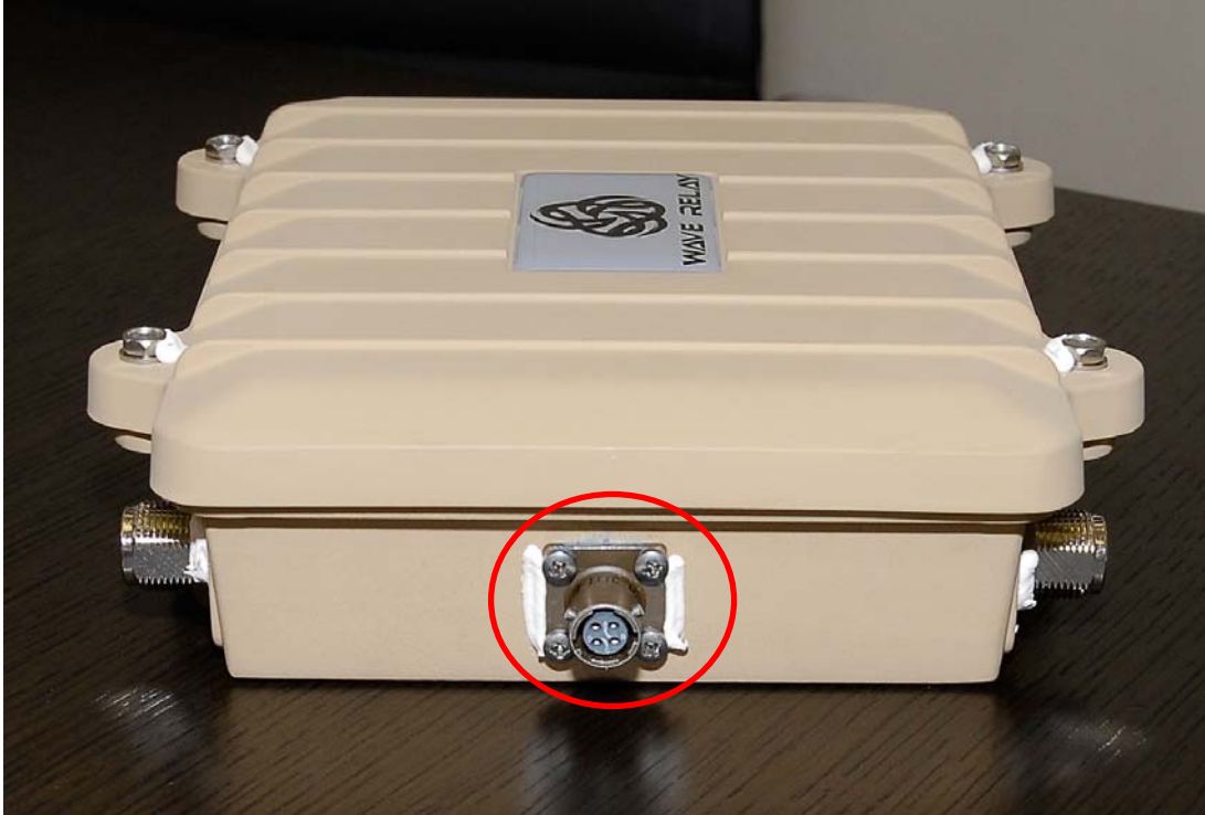
Figure 7 – Tamper-evident material placement for Quad Radio Router Serial Port (Left – 2 locations indicated by the red circle)
