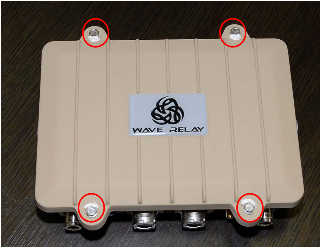
Figure 4 – Tamper-evident material placement for Quad Radio Router Cover (4 locations indicated by red circles)
