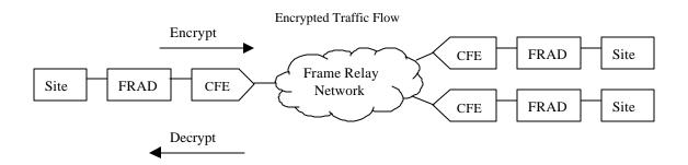
Secured connections are automatically established between the cryptographic module and similar units using a Diffie-Hellman key exchange process. This results in a separate secure link per connection and does not require any secret connection keys to ever be displayed or manually transported/installed. Secret connection keys will never leave the secure boundary in clear text form and they are not stored in non-volatile memory in clear text form.
