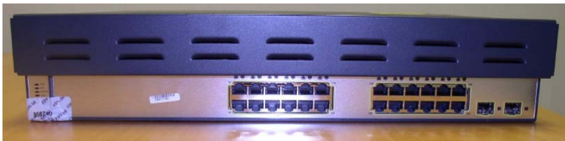
Figure 3 Placement of Tamper evident label on the cap of the mode button
