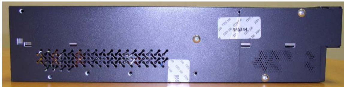
Figure 6 Placement of Tamper evident labels over the opacity shield and the removable cover
