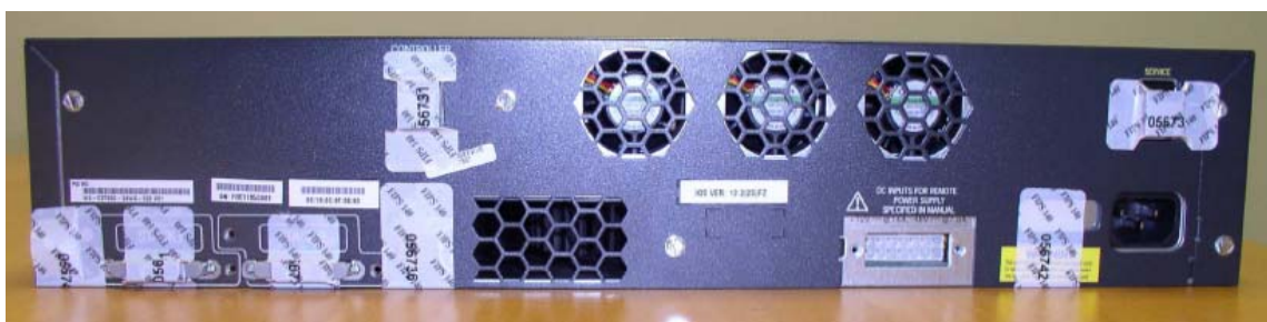
Figure 4 Placement of Tamper evident labels over the serial port, service port, and stack ports
