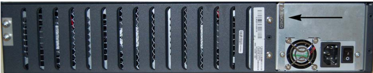
Figure 3: Rear of the SSG 520M and 550M devices, with location of tamper evident seal
