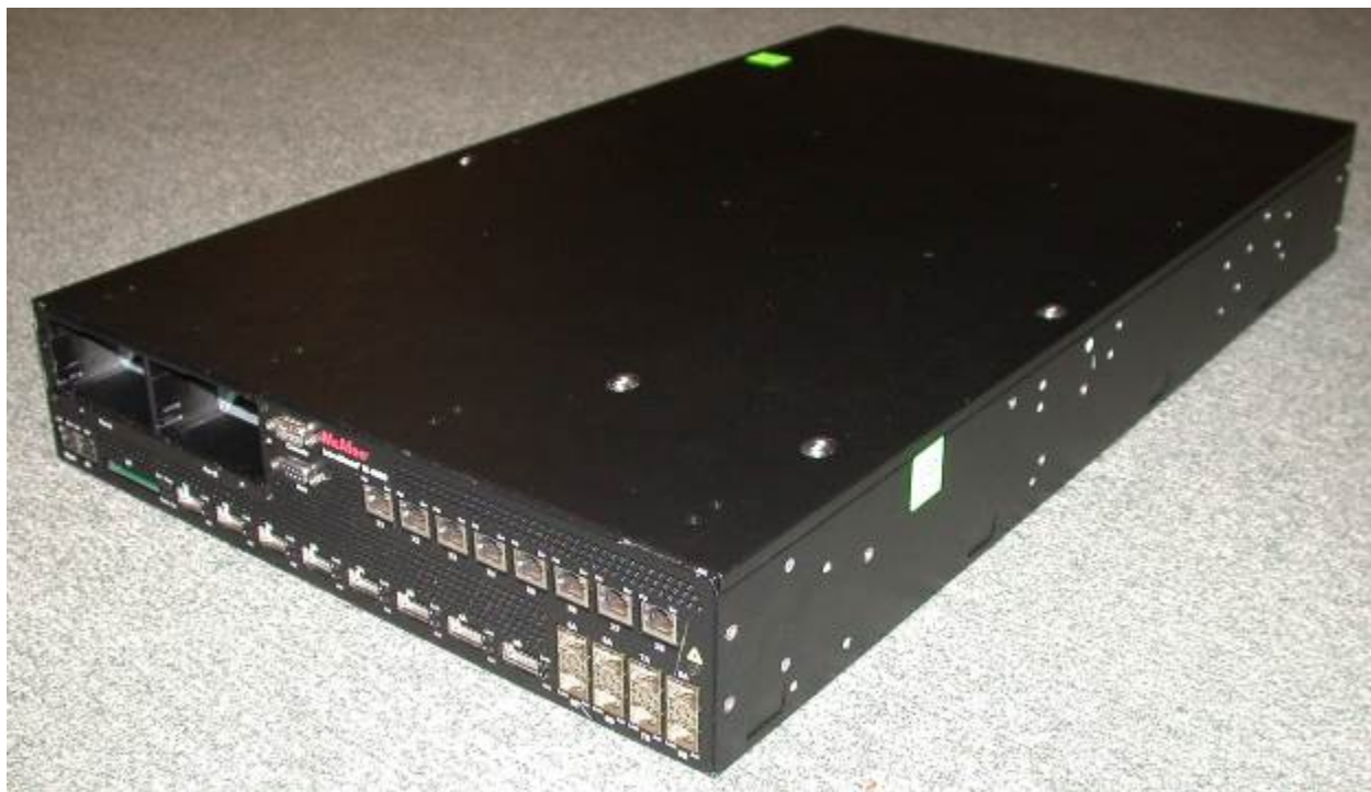
Figure 1 – Image of the Cryptographic Module (with Power Supply Trays Unpopulated)
