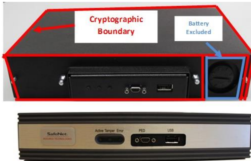
Figure 2-2. Luna G5 Cryptographic Boundary (with front bezel removed)
