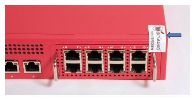
Figure 9: WatchGuard XTM 850, 860, 870 Front Panel Tamper Evident Label Placement
