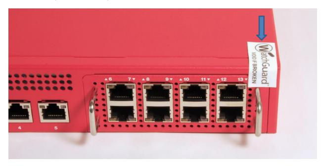
Figure 12: WatchGuard XTM 1520, 1520-RP Front Panel Tamper Evident Label Placement
